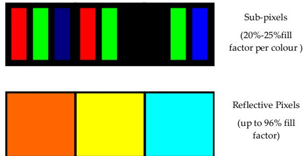
Figure 1: Pixel Fill factor
