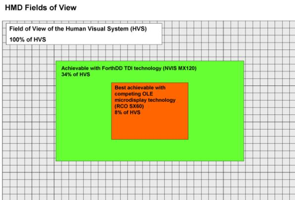
**Figure 3: HMD FOV vs. HVS FOV**
